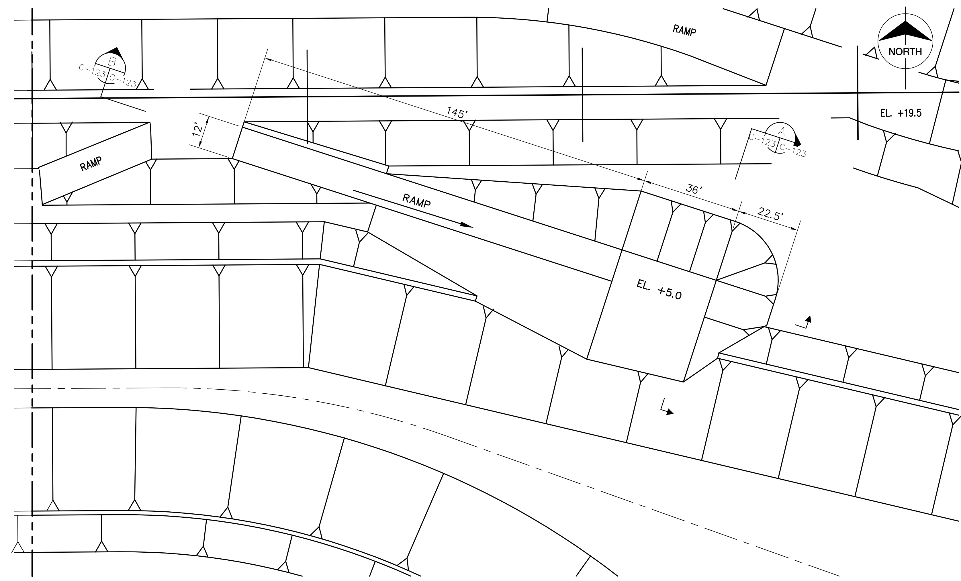
DISCHARGE SIDE BOAT LAUNCH DETAIL PUMP STATION G-370
